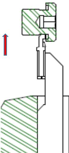
As Slide Continues to Feed, Draw Bar Shifts the tool into the Groove
