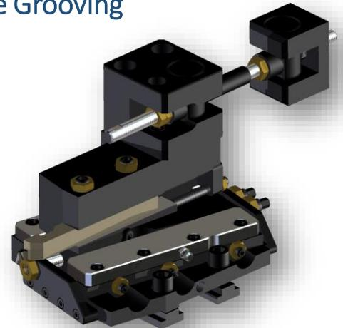
Tool Feeds Into the part from the cross slide
